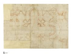
the grid could be used to relate explorative sketches of singular elements of the project, ranging in scale from the polygonal pillars to the general plan.
