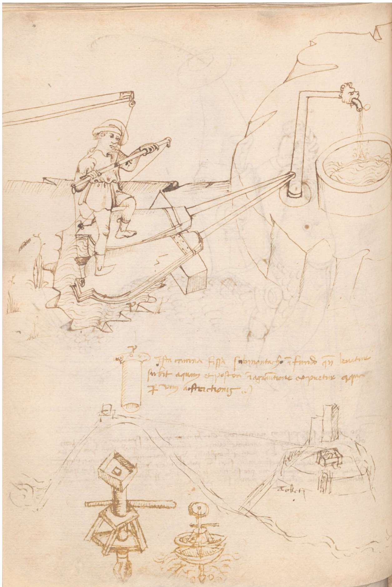
Mariano di Jacopo Taccola, double bellows used as water pump, siphon and boring devices, De Ingeneis (Books I & II) (Munich, Bayerische Staatsbibliothek, Codex Monacensis 197 II), fol. 31v.
